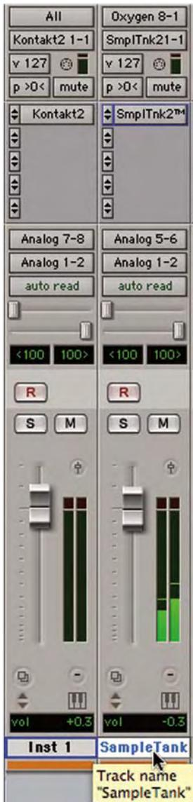
**Fig. 6.8** – Default Thru set to play the first selected MIDI track – in this case, SampleTank.
